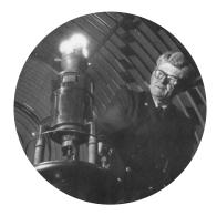
When the optic went into Mew Lighthouse, the fuel to produce the light was changed from gas to paraffin. The new paraffin lamps had three ceramic mantles which encased the flame and produced a bright white light equivalent to 1,210,000 candles.
